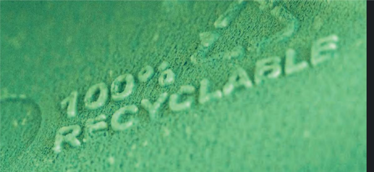
Material recycling is particularly suitable for materials such as paper or cardboard. Sorting and separation of various types of recyclable materials is the beginning of the process. The 100% recyclable paper injection molded packaging from our product portfolio is ideal for recycling because one of the main components of this environmentally friendly packaging is paper fiber.
