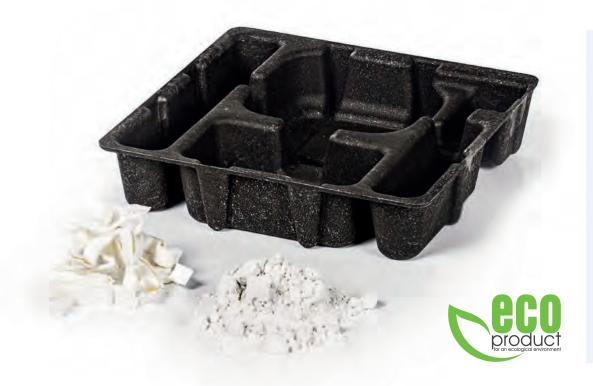
The renewable raw materials of reinpapier® paper mix include industrial starch (from industrial potatoes), long and short paper fibers, water, and an all-natural premix. The resulting paper mixture is then used for the injection molding process.
